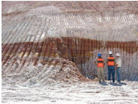
Figure 1. Kaolin ore containing lens with high concentration of red contaminant.
